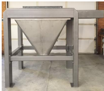
Hopper and Structure
